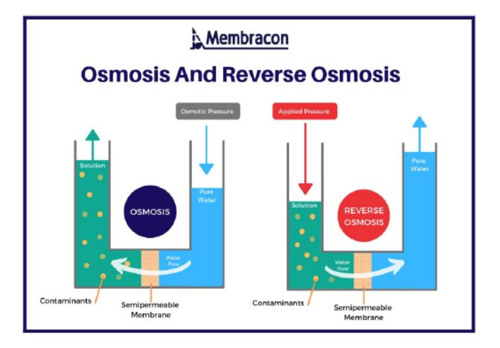
In osmosis, a lower-concentrate solution will filter its solvent to a higher concentration solution. In reverse osmosis, we are just reversing the process, by making our solvent filter out of our high concentrate into the lower concentrated solution.
